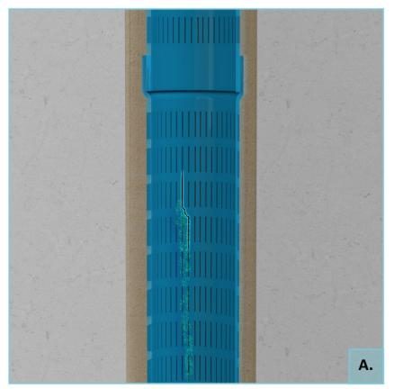
**A.** A visible crack in the well filter causes unwanted sand delivery and contamination. This well has become unusable and unreliable. Before the QRS can be inserted, the repair position should be determined with the necessary QRS length. It is also useful to have a caliber measurement for the ovality of the well (see above tolerances).
