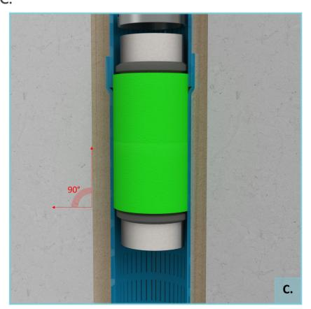
**C.** The QRS is placed over the crack and well (glue) connection. Unwanted sand deliveries and contaminations have now been remedied and the downhole tools can be retrieved. The installed QRS is aligned and placed at his right position. The system is repaired and ready for reliable use. The QRS is suitable for load forces about  $\pm$  <5.000 kg (diff. pres. <25bar).
