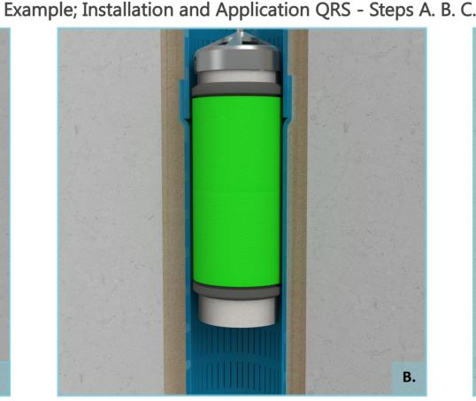
**B.** Insert the QRS at the intended position with universal downhole tools, supported by a winch or drilling-rig. The activation of the QRS starts when it comes into contact with the fluid. When the tool is at the damaged position, only some waiting time is required. The QRS will seal the position permanent, by the diffusion gradient between the QRS and motive fluid/water.
