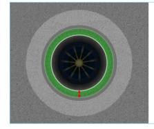
**BRIDGING COMPOUND** If the QRS comes into contact with the motive fluid, the compound activation will start. The swelling compound bridges the space between the well and QRS, with an increased volume of ± 1cm.
